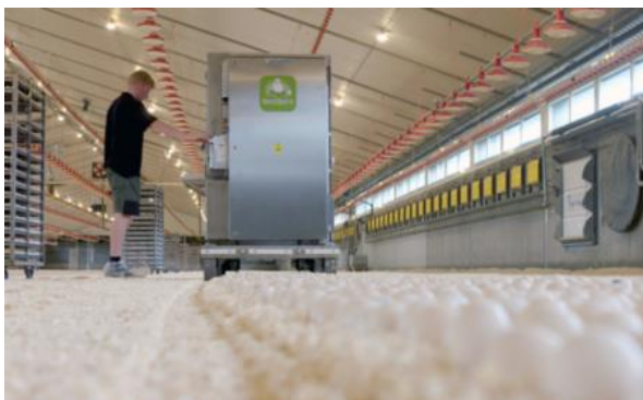
Fig.1: An egg placing machine places the incubated eggs directly in the litter bed at the farm. The capacity is 60,000 hatching eggs per hour. ©HFHC / NestBorn®
